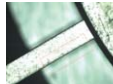
Positive edge detection with co-axial light
